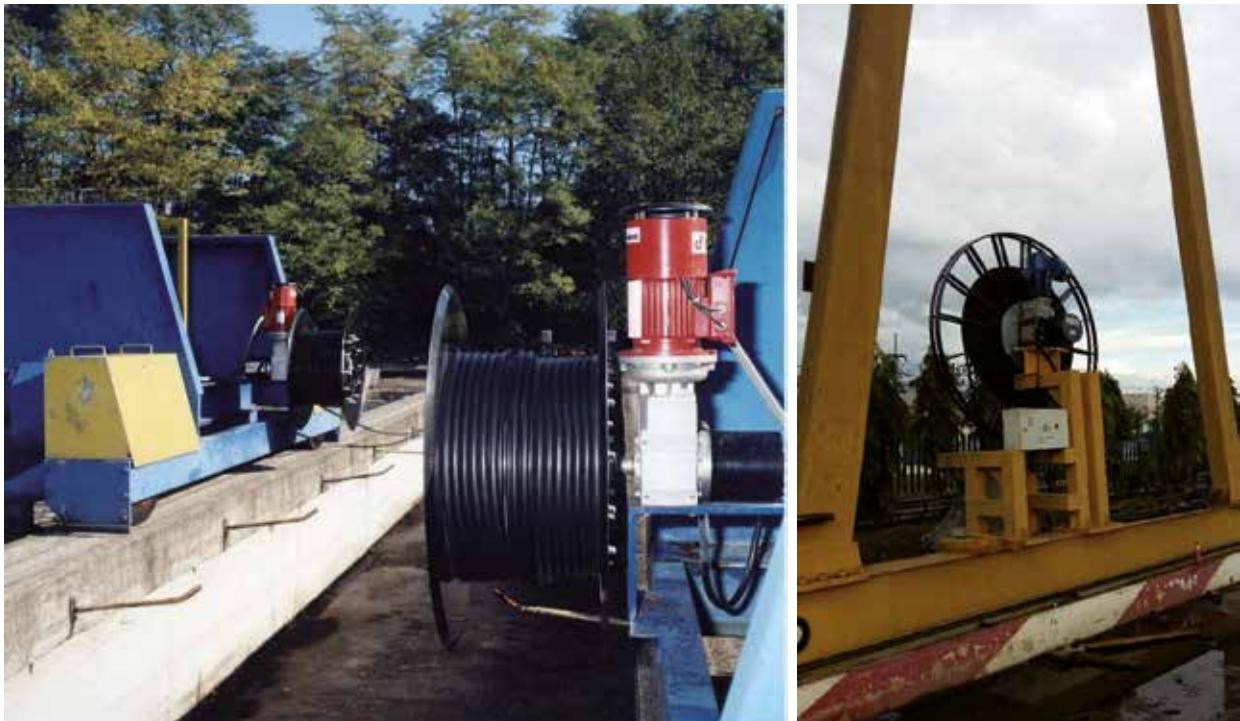
The Monospiral Spool wind the cable in the same plane and prevents the cable from twisting. It is your guaranty of a longer cable life. Monospiral Spools offer maximum exposure to ambient air and best cooling of the cable. The max reeling length is about 250 meter. The maximum diameter of the wheel is 3000 mm.
