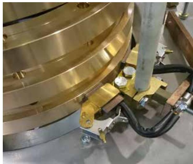
The slip-rings contacts are suitable for current transmissions from few mA up to 400 A, and rated voltage up to 0.6/1 kV. Special slip rings contacts are also used for data transmission, connecting PROFIBUS and PROFINET cables.
